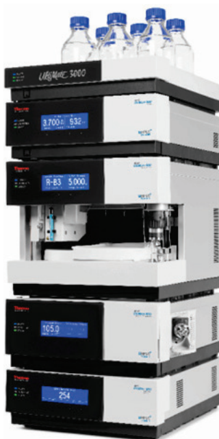
FIGURE 1. The UltiMate 3000 BioRS high-pressure, bioinert system.
