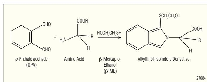
Figure 1. Derivatization of amino acids with OPA / β-ME produces electrochemically active thio-substituted isoindole.
