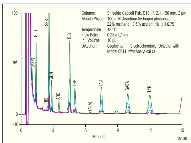
Figure 5. Overlay of four consecutive samples taken during the experimental time course.
