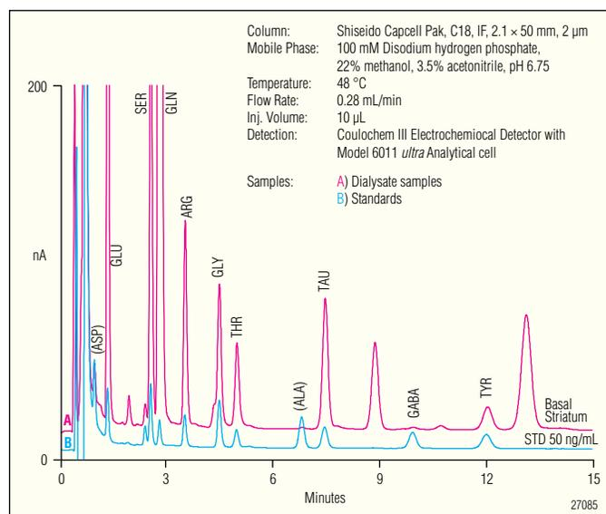
Figure 2. Overlay of amino acid analysis in samples and standard using 6011 cell.
