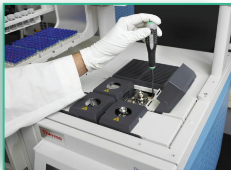
FIGURE 1. TRACE 1300 Series GC Modularity with user-installable modules
