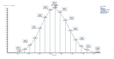
FIGURE 2. XIC of dieldrin (*m/z* 262.85642) showing 17 scans/peak (peak width 2.4 sec). Data acquired in full scan at 60,000 FWHM resolution (the exact resolution used is annotated in red). Mass accuracy/scan shown as ppm.
