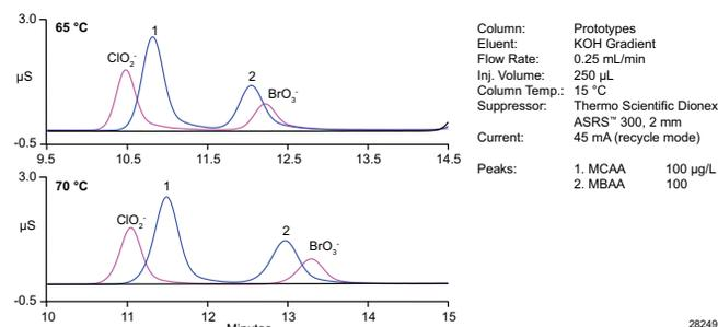
Figure 8 illustrates the separation using the new Dionex IonPac AS26 column. All nine haloacetic acid anions are separated from the matrix anions.
