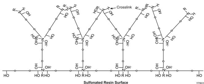
A new in-vial synthesis strategy was used for the Dionex IonPac AS26 columns. A basement layer was applied to the sulfonated resin by mixing the diepoxide/amine solution mixture (1:1 mole ratio of epoxide to amine) with the resin (sulfonated) at 70 °C for 60 min. This was functionalized by reacting the diepoxide with the resulting resin at 76 °C for 2 h then treating the resin with the same amine mixture solution at 76 °C for 1 h.
