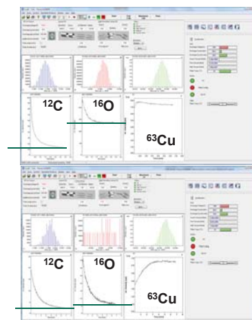
FIGURE 2. Carbon and Oxygen signal before (top) and after installation of moisture trap in the gas line (bottom).
