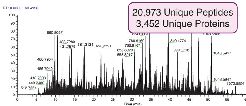
**FIGURE 2. Representative duty cycle. Each stick represents one scan, the first and last are full MS scans with MS/MS scans in between. The entire duty cycle took only 1.19 seconds, during which 1 full MS scan and 24 MS/MS scans were acquired.**
