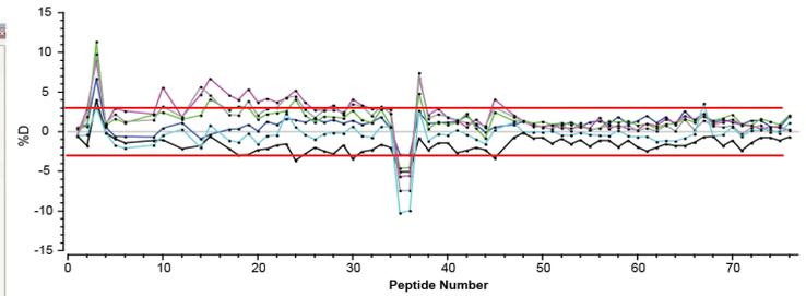
**FIGURE 7. Effect of labeling solution. Deuterium uptake residual plot of two different labeling conditions. Condition two showed more deuterium uptake than labeling condition one for all of the peptides measured.**
