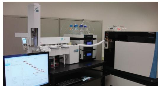
FIGURE 2. Components of H/D-X PAL
