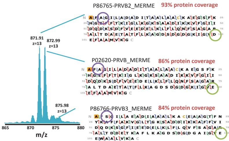
FIGURE 5. Full characterization of the three different main isoforms for the European hake. The high ion transmission at isolation widths down to 1 amu not only allows for high sensitivity that allows the identification and characterization of the three main isoforms, but also allows for high sensitivity, specifically in the case of PRVB3 which is the less abundant of the three of them. Circles in the amino acid sequence indicate the different substitutions.
