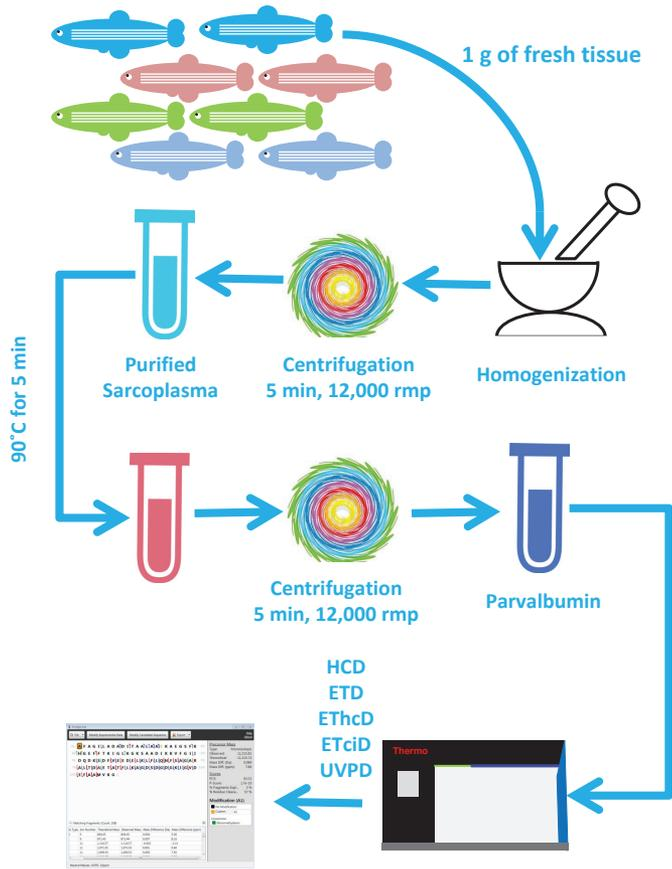
FIGURE 1. General overview of the analytical workflow. Reference muscle samples are processed. The thermo-stable proteins, beta-parvalbumins are purified and analyzed by top-down mass spectrometry
