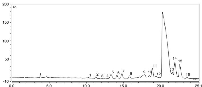
FIGURE 3B. Impurity Analysis of Apramycin with the SCX-UV Method.
