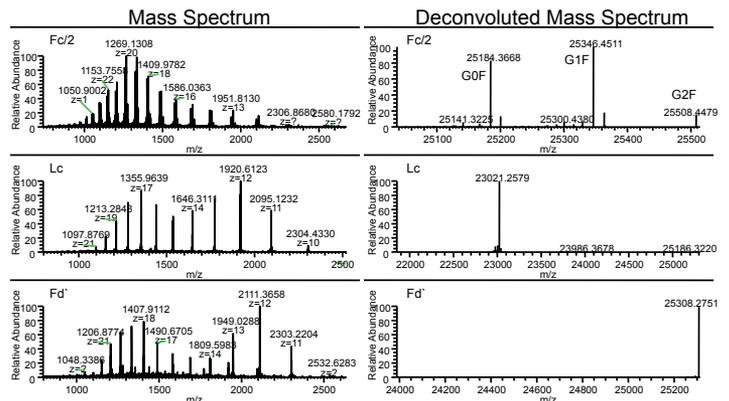
**Figure 9.** (Left) Mass spectra and (right) the deconvoluted mass spectra with molecular weights for Fc/2, Lc, and Fd' rituximab fragments for the corresponding peaks shown in figure 8.
