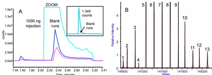
**Figure 7.** (A) TIC for 1000 ng injection and following 2 blank runs and (B) enlarged region of the deconvoluted spectrum showing low abundance glycoforms, see table 6 for masses.
