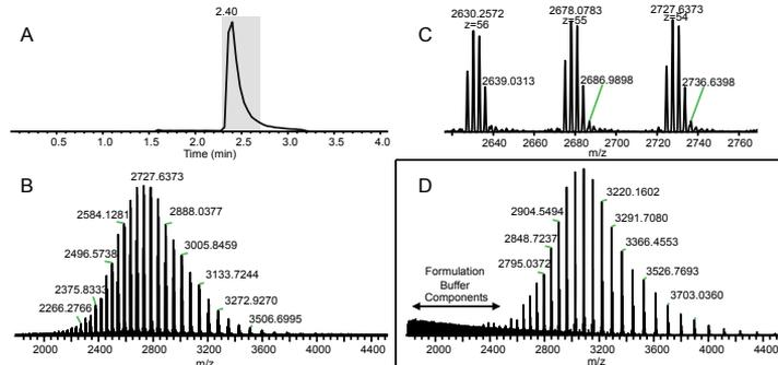
**Figure 5.** Loading, desalting and MS analysis of 100 ng rituximab: (A) Total Ion Chromatogram, (B) average full mass spectrum of gray region in (A), (C) enlarged region of mass spectrum showing 3 most abundant charge states, and (D) an example of poor desalting of a mAb performed on a 100  $\mu$ m x 250 mm C4 reversed phase column.
