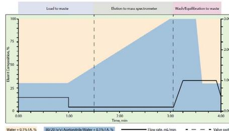
**Figure 3.** Schematic depiction of high throughput LC-MS method with dashed lines indicating divert valve switching.
