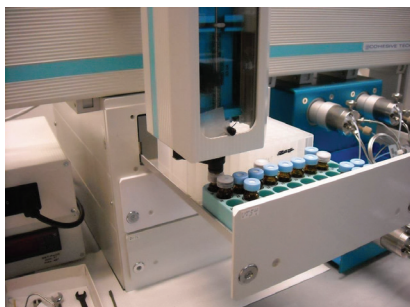
Figure 5. Autosampler objects – calibrate all positions
