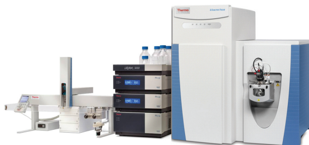
Figure 1. System configuration used for this work consisting on a Transcend II TLX1 system coupled to a Q Exactive Focus mass spectrometer.
