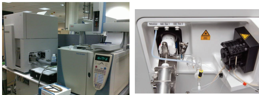
FIGURE 1. Picture of the TraceGC and TriPlus Autosampler hyphenated to the iCAP Q (left) and detail of the Dual Mode Interface (right).
