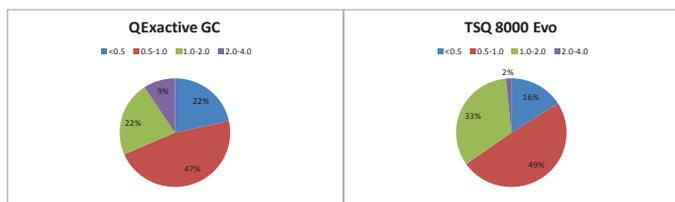
**FIGURE 4.** Comparison of the IDL<sub>99</sub> (ng/g) calculated for 132 pesticides from a 5 ng/g matrix-matched standard from the Q Exactive GC-MS (left) and TSQ 8000 Evo triple quadrupole GC-MS (right). Percentage of pesticides and corresponding IDL interval relative to the total number of target compounds (132) is indicated.
