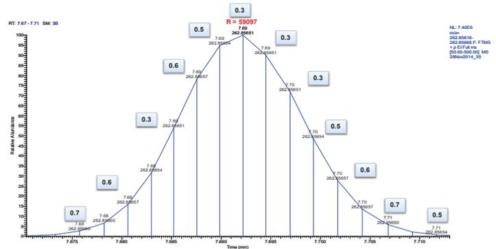
FIGURE 2. XIC of dieldrin (m/z 262.85642) showing 17 scans/peak (peak width 2.4 sec). Data acquired in full scan at 60,000 FWHM resolution (the exact resolution used is annotated in red). Mass accuracy/scan shown as ppm.
