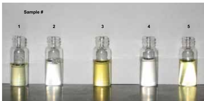
FIGURE 6. Five lots of Polysorbate 80 illustrating various physical properties in different vendor products.
