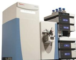
Thermo Scientific™ Q Exactive™ Plus mass spectrometer with a Thermo Scientific™ UltiMate™ 3000 RS UHPLC system
