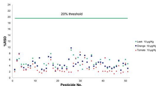
The results of the 10 replicate injections at 10 µg/Kg in all three matrices are presented in Figure 10. All of the detectable pesticides had RSD% less than 10%, well below the 20% threshold requirement in the SANTE guidance document. This shows that the system has the selectivity and sensitivity required to analyse pesticides in a robust manner at the MRL.
