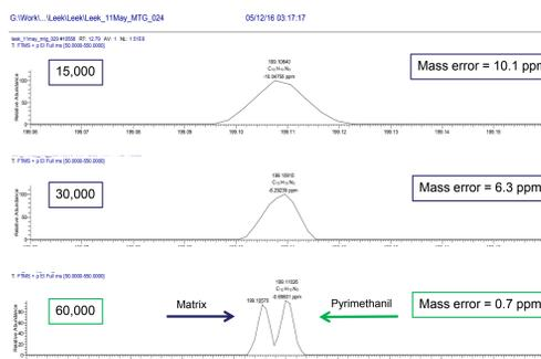
Figure 6. Mass difference measurements at the LOI level for each pesticide across the three matrices.
