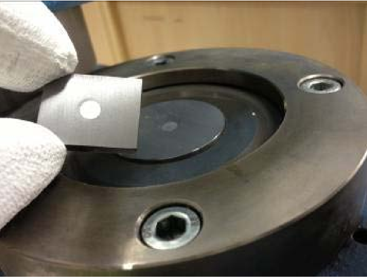
FIGURE 1. Alumina pellet pressed into high purity tantalum target acting as a secondary electrode.
