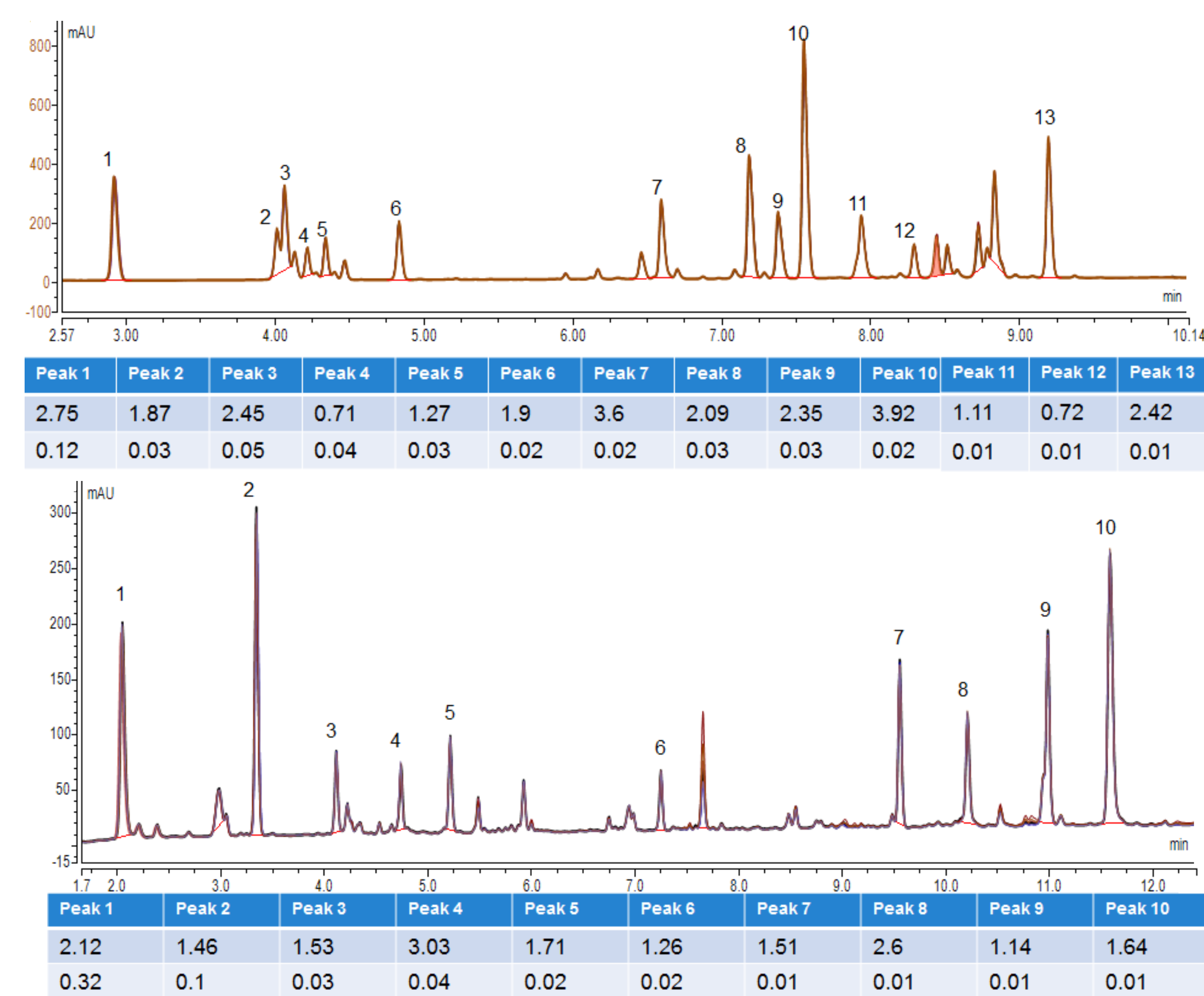
Figure 2. Automated digestion of Cytochrome C and carbonic anhydrase using SMART Digest magnetic resin with the KingFisher Duo Prime system. Overlaid peptide maps of different digests of Cytochrome C (upper panel) and carbonic anhydrase (lower panel). Digest solutions were injected without further purification. %RSD values for relative peak area (upper) and retention time (lower) and are given for the peaks indicated.
