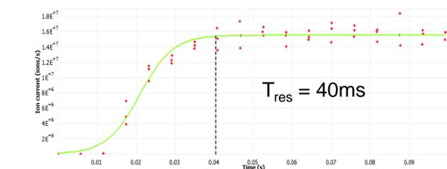
Figure 10. CV Switching Time Plot for TSQ Altis Equivalent Transfer Tube
