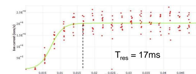
Figure 11. CV Switching Time Plot for TSQ Quantiva Equivalent Transfer Tube
