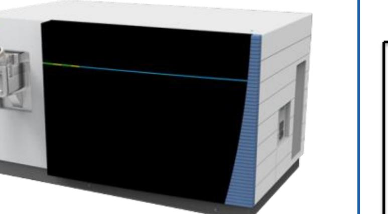
The Thermo Scientific™ Pierce™ Intact Protein Standard mix was also analyzed with an Orbitrap Fusion Lumos Tribrid mass spectrometer, which we coupled to a Thermo Scientific™ Dionex™ UltiMate™ 3000 ultra-high pressure LC operating at 2000/min. We analyzed the sample with a data-dependent method that consisted of a 15k resolution (@200m/z) Orbitrap MS1 scan followed by data-dependent Orbitrap MS2 scans with the precursor charge state filter set to ≥+7.
