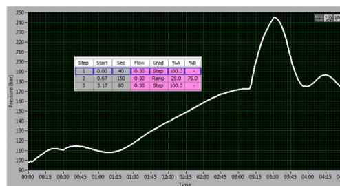
**Figure 3. PFP column pressure trace showing sufficient equilibration.**
