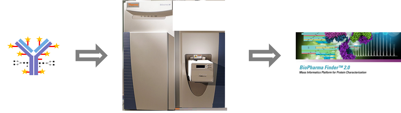
FIGURE 6: Workflow 2: Lysine-linked ADC analyzed by ZipChip based electrophoresis coupled to a Q Exactive HF and processed with BioPharma Finder 2.0
