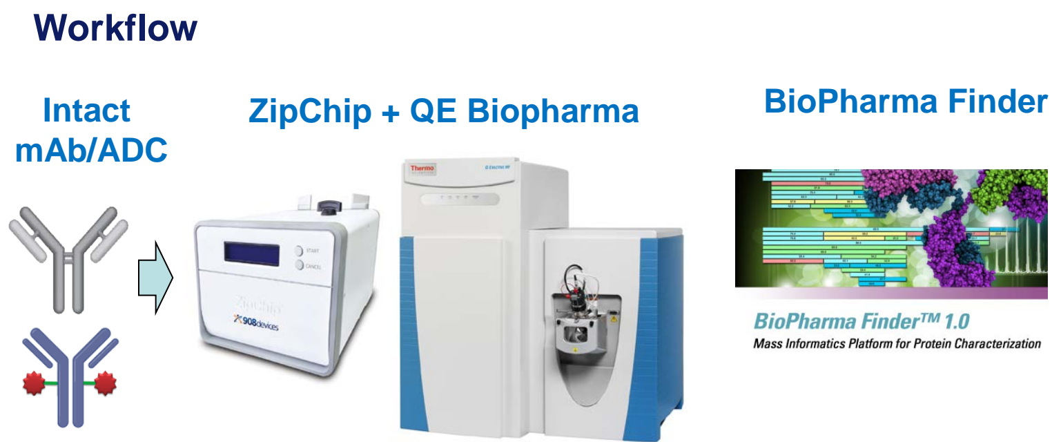
Figure 1. Characterization of mAb/ADC is accomplished by separation with the ZipChip device, on-line analysis with high resolution Q Exactive Biopharma mass spectrometer, and identification with BioPharma Finder software.
