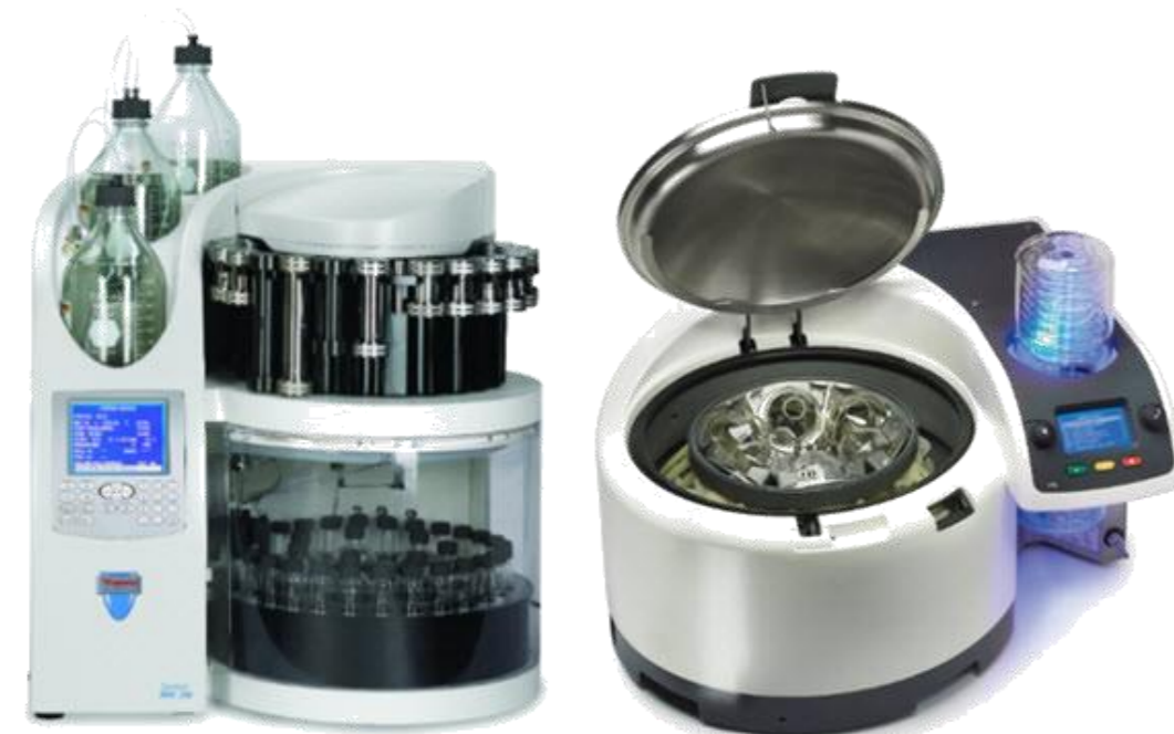
FIGURE 2. Thermo Scientific Dionex ASE 350 and Thermo Scientific Rocket Evaporator system
