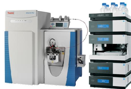
FIGURE 1. Thermo Scientific Q Exactive Plus mass spectrometer with Thermo Scientific Ultimate 3000 HPLC
