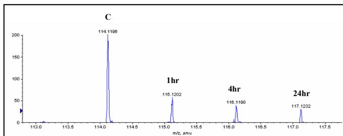
MS/MS region revealing iTRAQ™ reagent quantitation tags from the kit peptide fragmentation spectra shown in Figure 2. Fragment ion spectra of kit peptide from 4-plex labeled anti-pY sample following 1, 4 or 24 hours exposure to Kit/KDR inhibitor or control (C).
