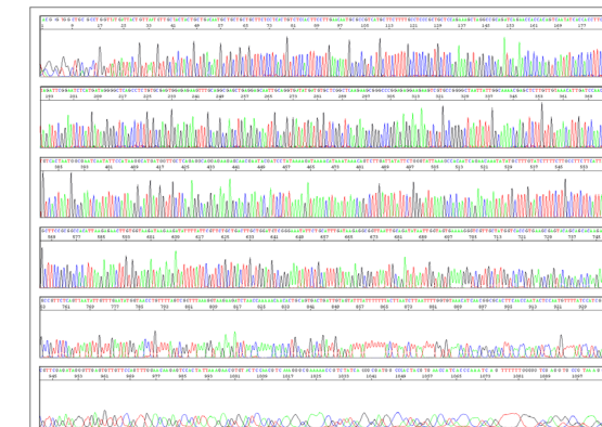
Figure 4. This electropherogram from a 3130x/ Genetic Analyzer is an example of a typical long-read sequence obtained from a BigDye Terminator Sequencing Standard v3.1. A QV 20 LOR of 1,090-bp was achieved using 3130 POP-7 polymer. Total run time: 2 hr, 50 min.
