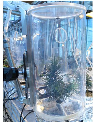
Figure 4. Transparent gas-exchange chamber with pine seedling
