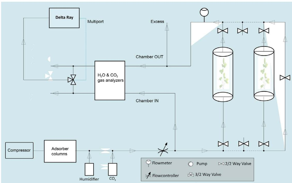
Figure 5. Simplified schematic of the plant gas exchange set-up with the Delta Ray IRIS included. Measurements were conducted in a scientific greenhouse at KIT/IMK-IFU, Garmisch-Partenkirchen, Germany.
