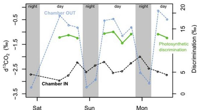
Figure 6. Time series of averaged  $\delta^{13}\text{CO}_2$  for air entering (chamber IN) and air leaving (chamber OUT) a plant chamber. Photosynthetic discrimination is given during daytime, calculated from the differences in  $\delta^{13}\text{CO}_2$  and  $\text{CO}_2$  concentrations of chamber IN and chamber OUT.
