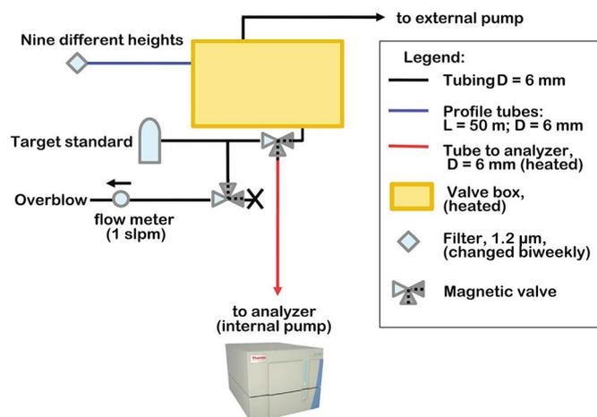
Figure 2. Simplified schematic of the monitoring setup in the beech forest
