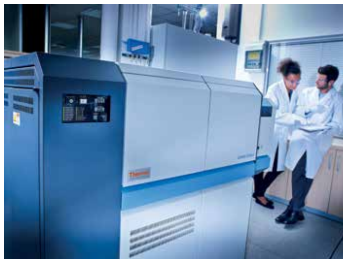
Figure 2. The Thermo Scientific Element GD Plus GD-MS.
