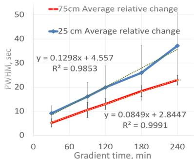
**Figure 4. Estimated peak capacity as a function of gradient length for 25 cm and 75 cm x 75 μm EASY-Spray columns**
