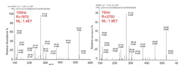
**Figure 5. MRFA mS/MS spectra at 75 and 100Hz (4 and 4ms transients).**
