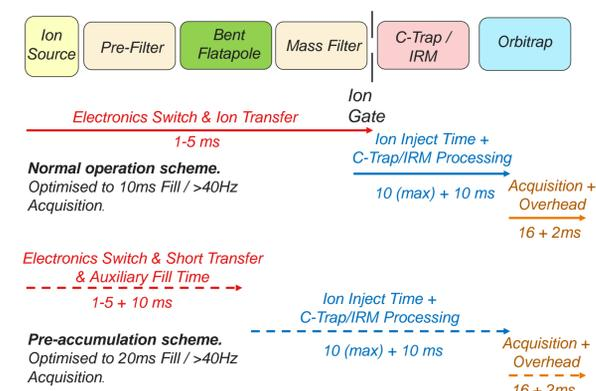
**Figure 1. Ion optical layout of an Orbitrap Exploris mass spectrometer, and illustration of in-series and in-parallel instrument operations in 40Hz standard and pre-accumulation modes.**
