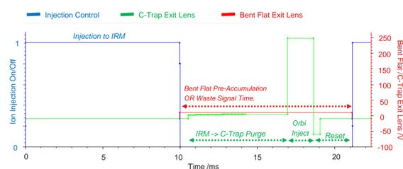
**Figure 2. Pseudo-oscilloscope plot during operation showing instrument event timing, including implementation of bent flatapole pre-accumulation.**
