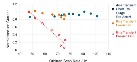
**Figure 4. Relative MRFA ion current with increasing repetition rate (decreasing inject time), for pre-accumulation active and disabled, for 8ms and 4ms orbitrap transients.**
