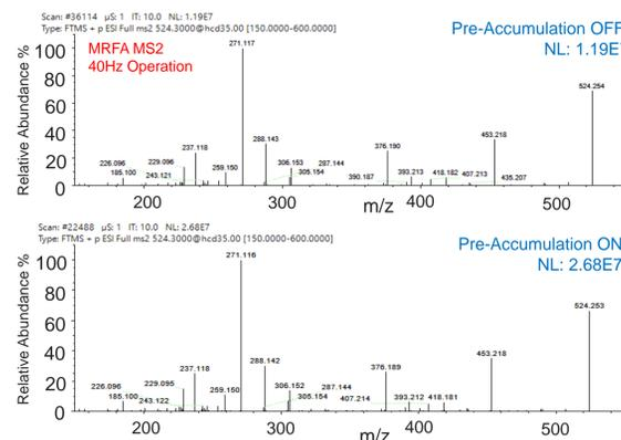
**Figure 2) Comparison of MRFA MS/MS spectra with pre-accumulation disabled (top) and enabled (bottom).**
