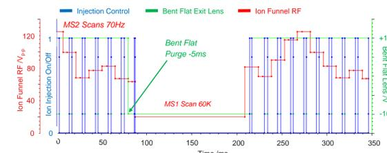
**Figure 6. Pseudo-oscilloscope plot of key events during MS and MS/MS scanning of a 70Hz Pre-Accumulation DDA Method.**
