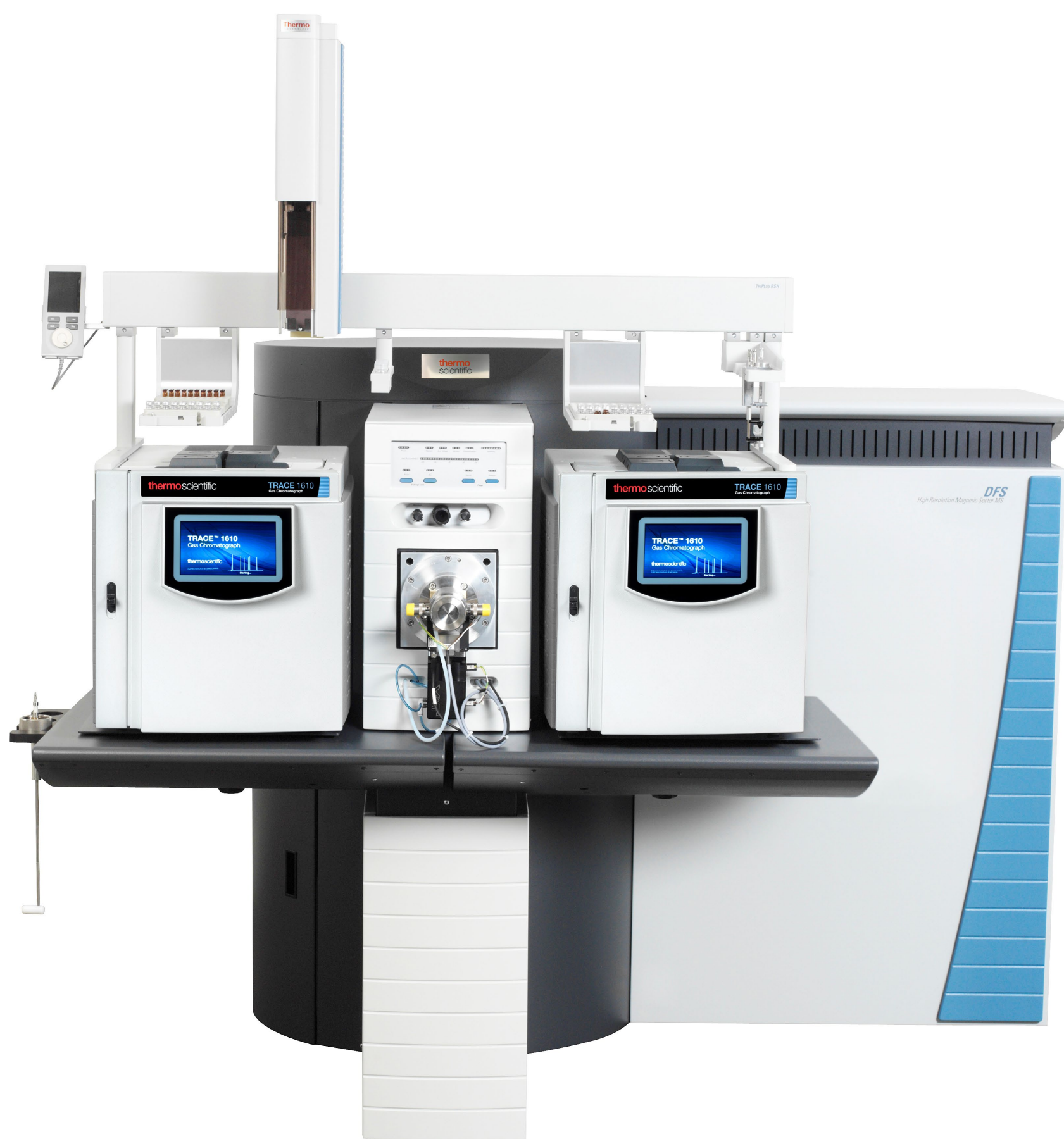
Figure 1. DFS Magnetic Sector GC-HRMS coupled to two TRACE 1610 GCs.
