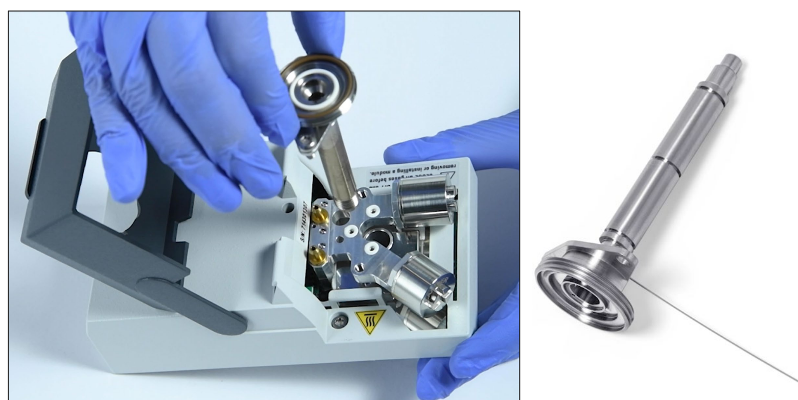
Figure 3. Exchanging the injector body of an SSL injector module with the HeSaver-H 2 Safer injector body (right side)
