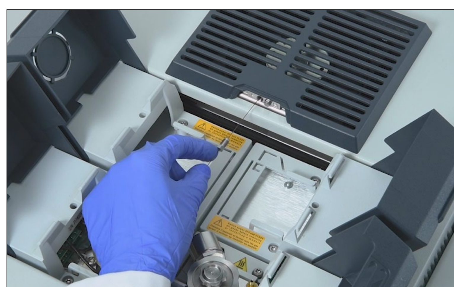
Figure 4. Installing the SSL Module with the HeSaver-H 2 Safer module and connecting the Helium gas tube.
