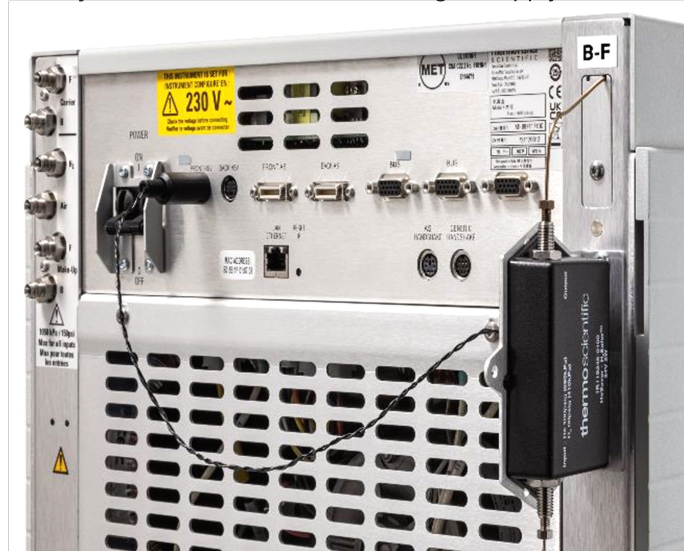
Figure 2. Valve module installed at the back of a TRACE 1610 GC.
