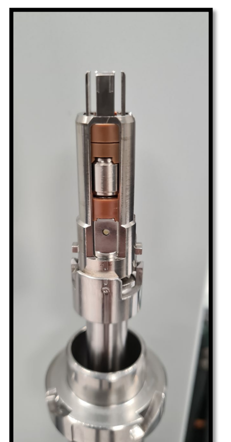
Ion source after 100 injections of raw soil extract
