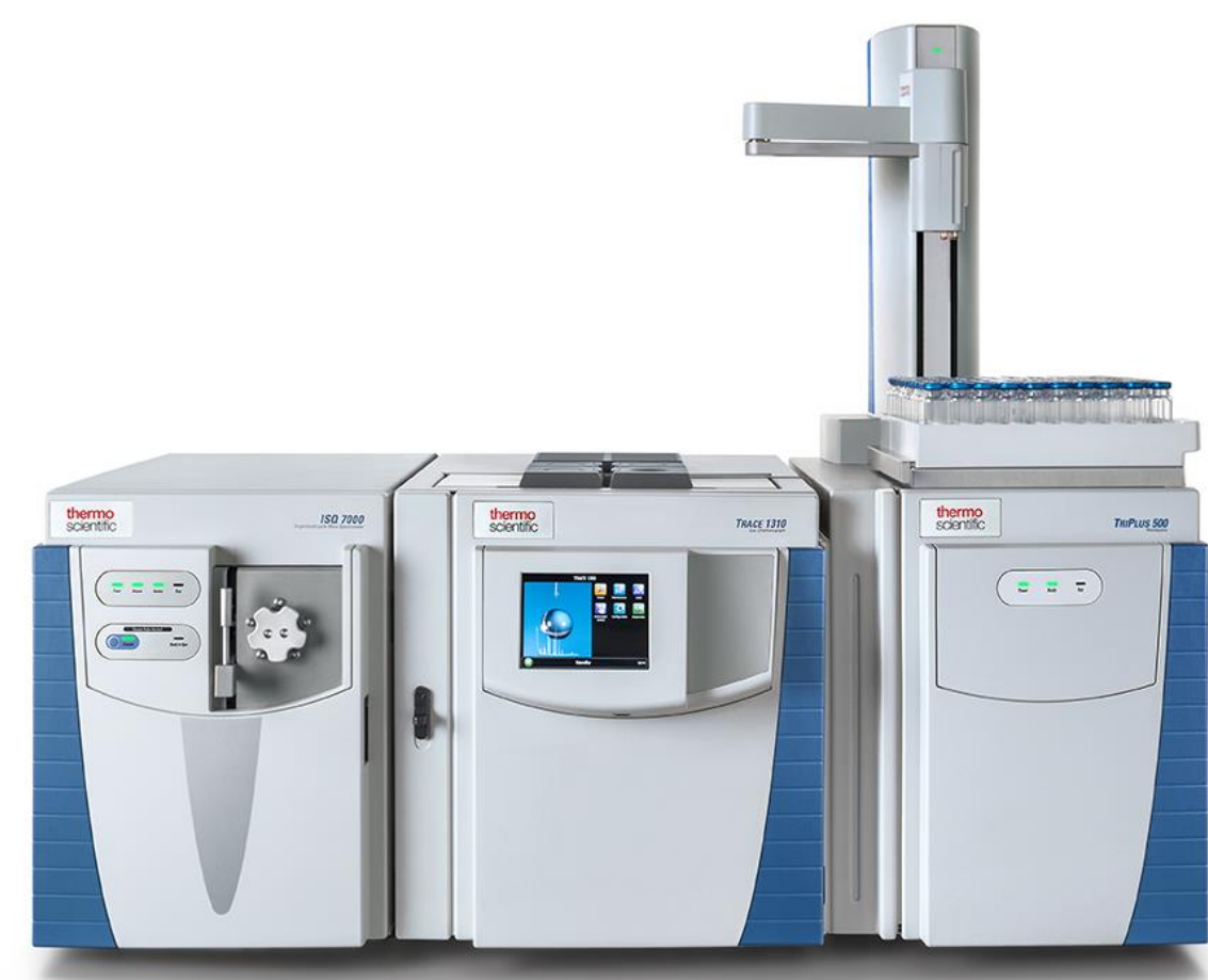
Figure 1. TriPlus 500 HS Autosampler coupled to a TRACE 1310 GC and ISQ 7000 Single Quadrupole MS.
