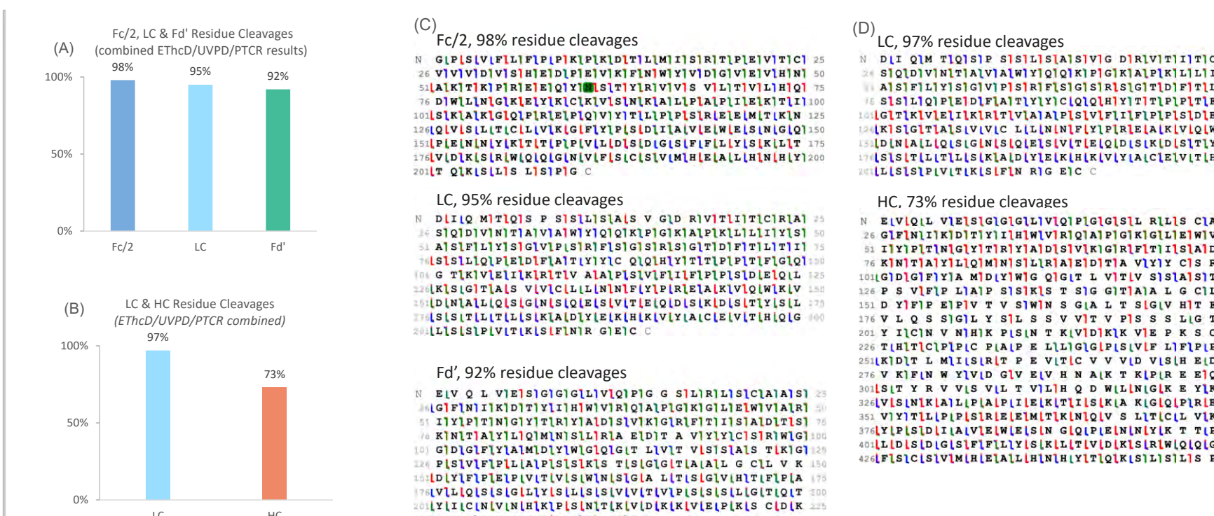
Figure 9. Combined results of ETHcD, UVPD, and PTCLR middle-down analyses provided excellent sequence coverage of trastuzumab subunits. A.) Bar chart showing a nearly complete sequence coverage of Fc/2, LC and Fd' subunits obtained from the combined results of ETHcD, UVPD and PTCLR raw files (10 in total); B) Bar chart showing a nearly complete sequence coverage of the LC subunit (97%) and high sequence coverage of the HC subunit (73%) when combining the raw files of ETHcD, UVPD and PTCLR (10 in total); C) Fragmentation maps of the Fc/2, LC and Fd' subunits from the combined results of 10 raw files; D) Fragmentation maps of the LC and HC subunits from the combined results of 10 raw files.
