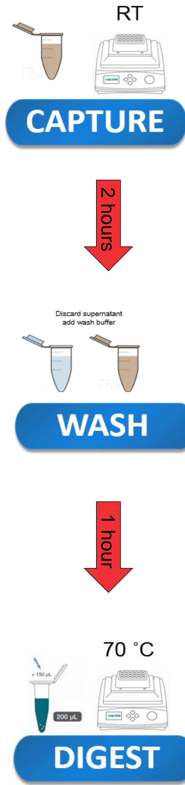
Figure 4: Three step process, all carried out on the same bead, for capture, wash and digestion of target mAb.
