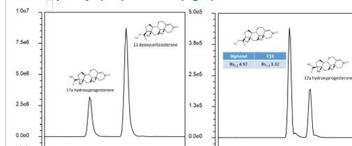
Figure 4. Separation of structural isomers 17 $\alpha$ -hydroxyprogesterone and 11-deoxycorticosterone on biphenyl (left) and C18 (right), both with m/z 331.2
