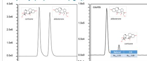
Figure 5. Separation of structural isomers cortisone and aldosterone on biphenyl (left) and C18 (right), both with m/z 361.2
