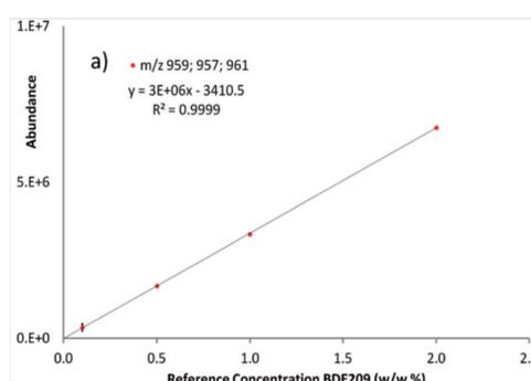
Figure 3. Calibration curves and linearity for the analysis of (a) [BDE209]+, (b) [BDE209-Br<sub>2</sub>]+ obtained by DIP.
