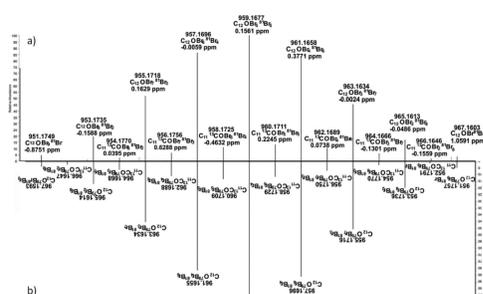
Figure 2. Comparison of (a) accurate masses measured over 20 scans for BDE209 and (b) their calculated exact value.
