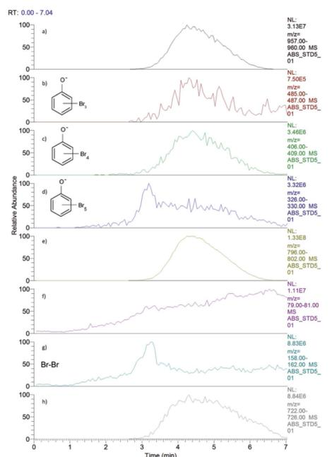
Figure 4. Time signal obtained with DIP-HRMS. penta brominated ions (d) corresponds to a simultaneous release of Br<sub>2</sub> molecules (g).
