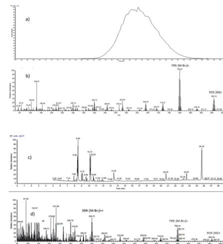
Figure 5. TIC and mass spectra for RM (ABS with 0.5% BDE209) (a-b) DIP-HRMS, (c-d) GC-MS.
