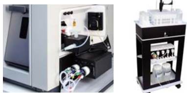
FIGURE 1. prepFAST connected to the iCAP Q (left), ESI SC-2DX autosampler (right).
