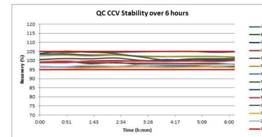
Figure 3. QC CCV Stability Data Over 6 Hours.
