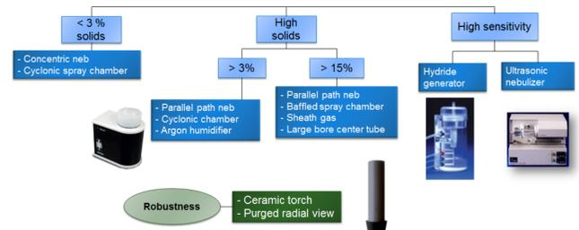
Figure 1. Aqueous sample introduction recommendations.
