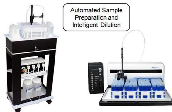
Figure 2. ESI prepFAST (left) and CETAC SDX High Performance Liquid Dilution System (HPLD) (right).
