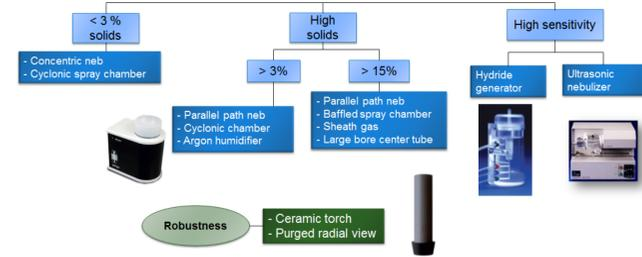
Figure 1. Aqueous sample introduction recommendations.
