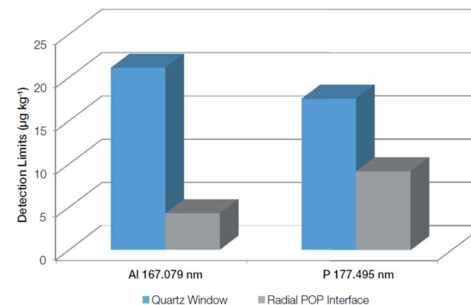
Figure 4. Improved detection limits of Al 167.079 nm and P 177.495 nm in the radial view of a dual view iCAP 7000 Plus Series ICP-OES Analyzer.
