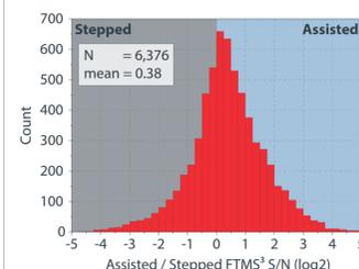
Figure 9. When 6,376 matching FTMS<sup>3</sup> spectra were compared between Stepped and Assisted HCD on the Ginseng extract, the average signal-to-noise of the FTMS<sup>3</sup> spectra increased ~30% when using Assisted HCD for the MS<sup>2</sup> stage.
