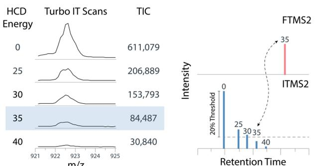
Figure 2. Assisted CE scan for precursor 923.01 m/z using 4 energies (25, 30, 35 and 40). The optimal collision energy of 35 was selected by the instrument as having reduced the precursor below the 20% threshold.
