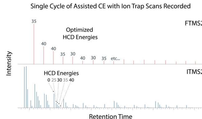
Figure 3. A single MS-MS/MS cycle using assisted collision energy acquisition results in the analytical FTMS<sup>2</sup>s using a range of collision energies.
