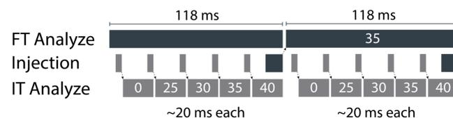
Figure 4. Pipelining of the ion trap scans for assisted collision energy determination with 60K FTMS<sup>2</sup>s. The five ion trap injections and analyses can occur during the preceding FT transient period and are used to calculate the optimal energy for the next FT injection and analysis step.
