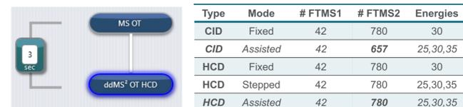
Figure 5. The effect of assisted collision energy on the duty cycle of an MS/MS experiment using different collision energy modes. The slight decrease in CID assisted mode is due to the CID activation time (10 ms) adding an appreciable amount of time to the hidden ion trap scans.
