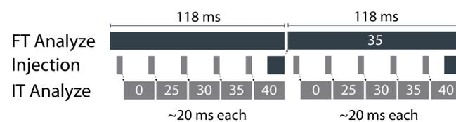
Figure 4. Pipelining of the ion trap scans for assisted collision energy determination with 60K FTMS<sup>2</sup>s. The five ion trap injections and analyses can occur during the preceding FT transient period and are used to calculate the optimal energy for the next FT injection and analysis step.
