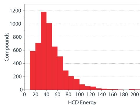
Figure 1. Distribution of optimal HCD energies for 5,575 compounds in the mzCloud database. Optimal energy is determined by the MS<sup>2</sup> spectrum with the most intense fragment ion current. The mean HCD energy was 43±27 NCE and shows that optimal fragmentation conditions are highly compound-specific.
