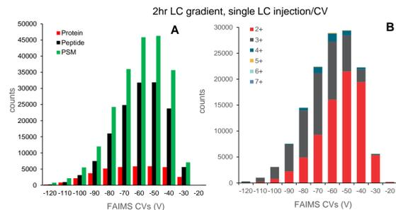
CVs -90V to -40 contained the most PSM counts and yielded the most peptide/protein IDs (left). This correlated with the charge state distribution histogram (right) that showed the same CV range enriched with multiply charged species (2+ to 7+). There was also correlation between charge state and CV bins; for example -50V was dominated by 2+ and -70V -80V was dominated by 3+. This shows how charge enrichment occurs in FAIMS CVs and helps selection of CVs for a DDA.
