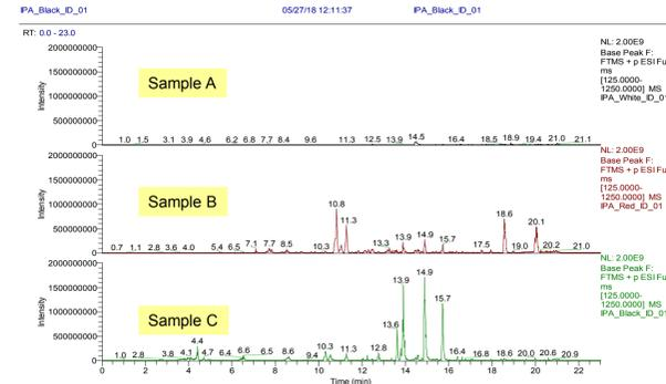
The constant presence of solvent background often masks the low-abundant additives in the extracts solution. By using the AcquireX background exclusion workflow, several sulfur-containing additives were readily identified, which are substances of concern.
