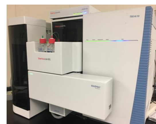
TSQ Altis mass spectrometer mounted with FAIMS Pro interface and VeriSpray source
